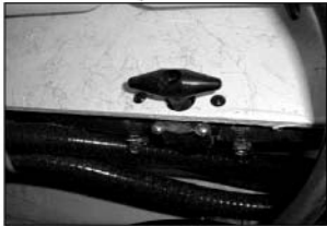
Fish box drain valve on models 2180, 2300. Located in battery compartment
