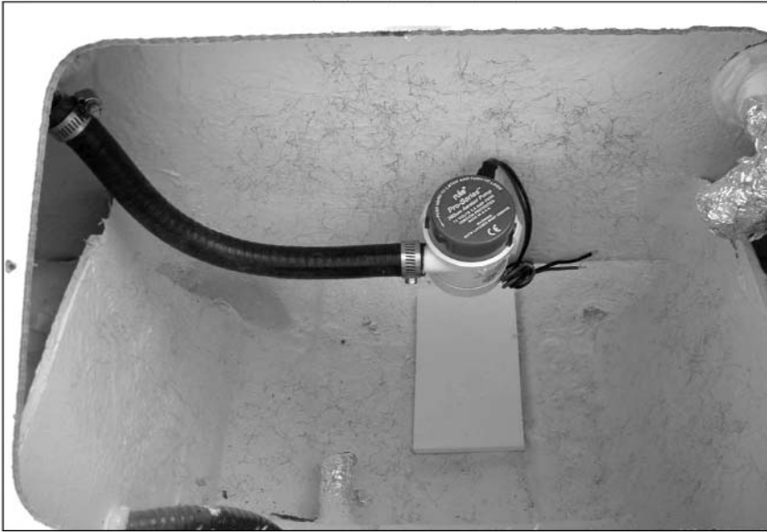
Fish box drain valve on models 2180, 2300. Located in battery compartment
